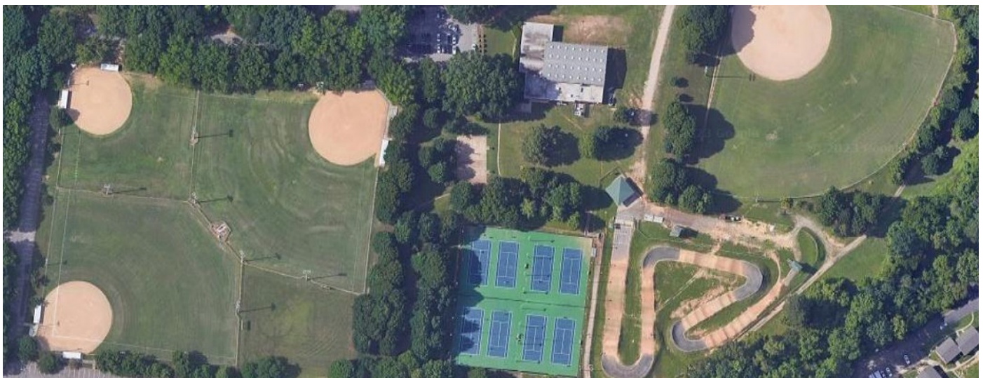
FIGURE 6. Accounting for sports fields and lawns is important when characterizing natural areas using permeable surface data. The park shown below has 89% permeable surface, but almost all of that is due to sports fields.
